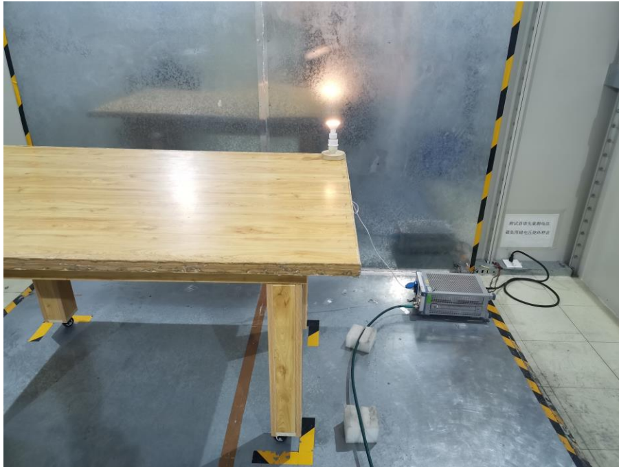
Conducted Emissions (Side View)
