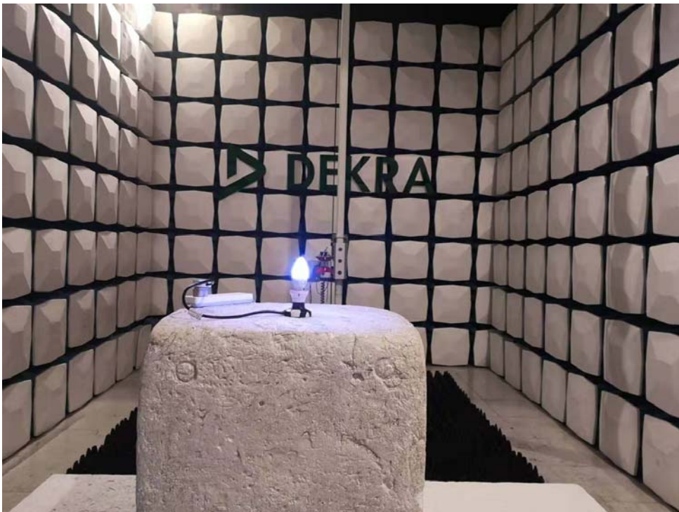
Description: Radiated Emission Test Setup for 1~18GHz
