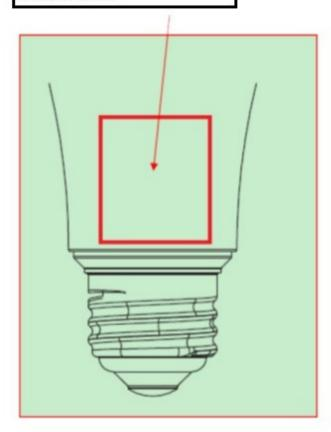
The label is indicated in exterior of the device and it is always visible without using any tool.
