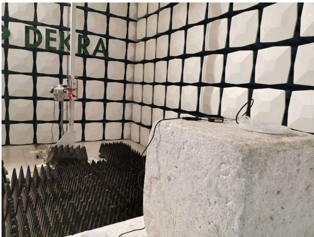
Description: Radiated Emission Test Setup for 1~18GHz
