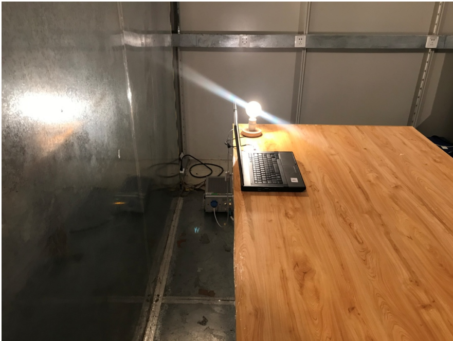
Conducted Emissions (Side View)
