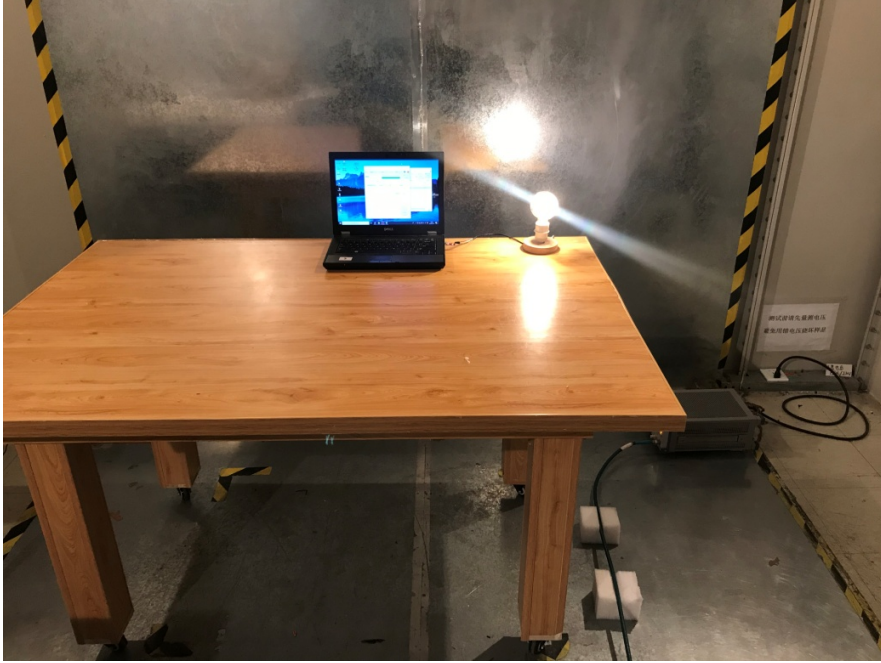
Conducted Emissions (Side View)
