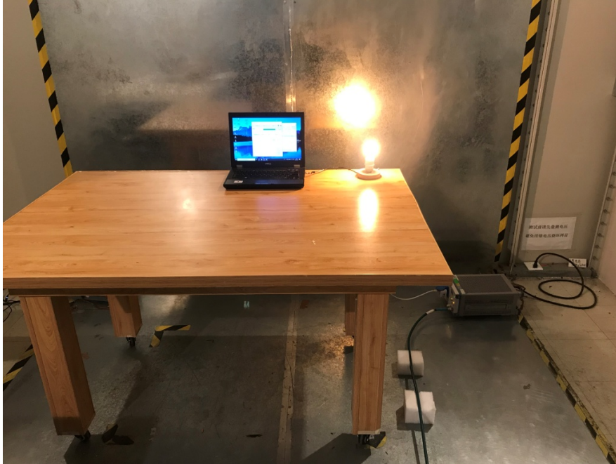
Conducted Emissions (Side View)
