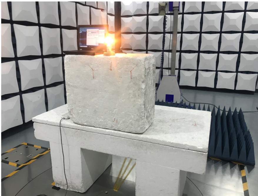
Radiated Emissions View(Above 1GHz)
