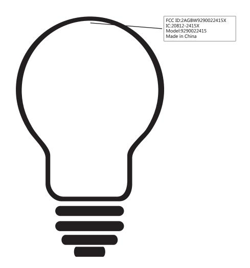
The label is indicated in exterior of the device and it is always visible without using any tool.
