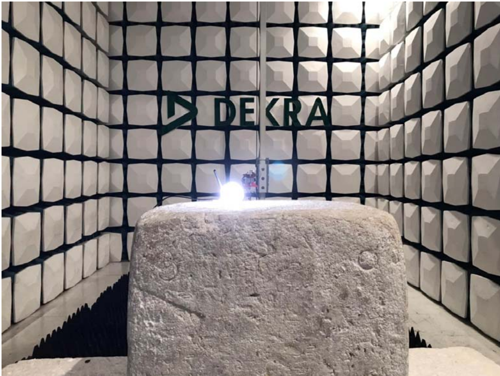
Description: Radiated Emission Test Setup for 1~18GHz
