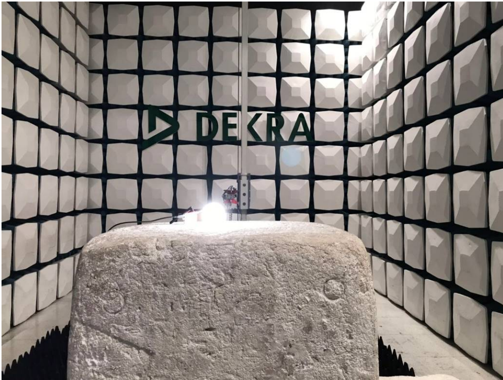
Description: Radiated Emission Test Setup for 1~18GHz
