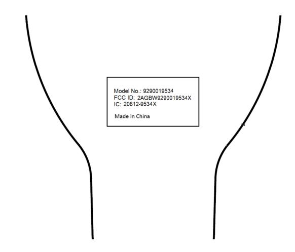
The label is indicated in exterior of the device and it is always visible without using any tool.
