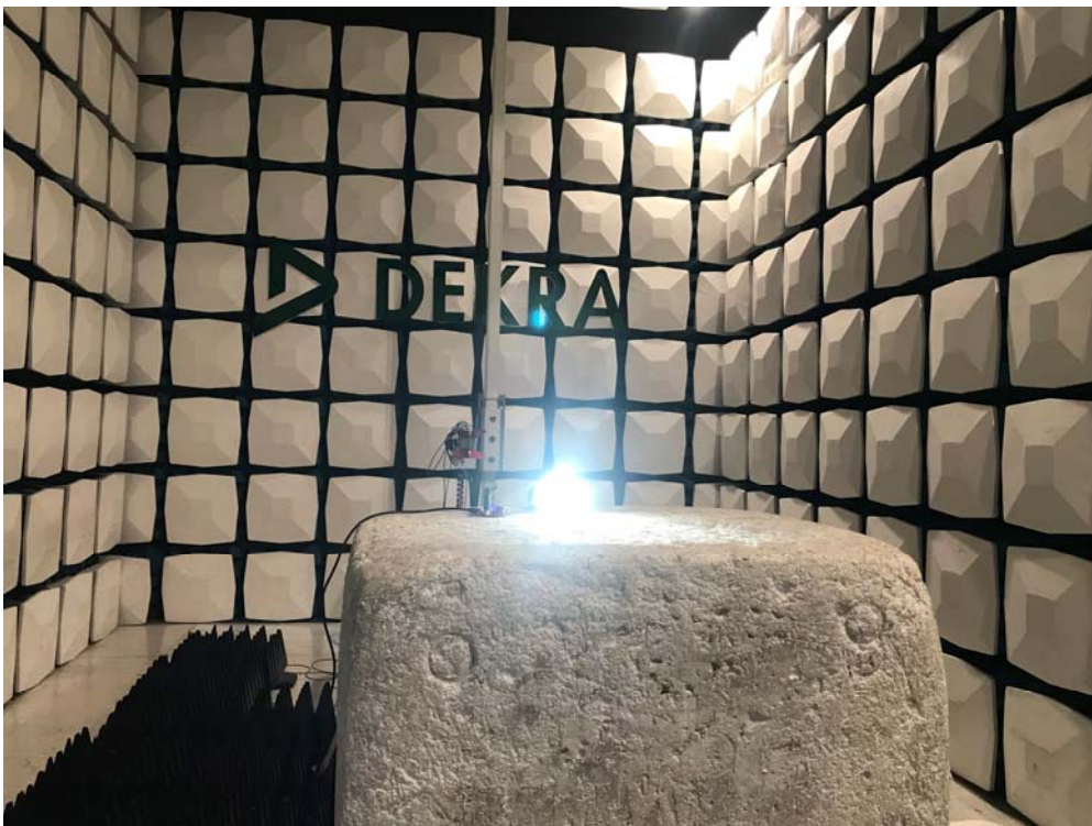
Description: Radiated Emission Test Setup for 1~18GHz
