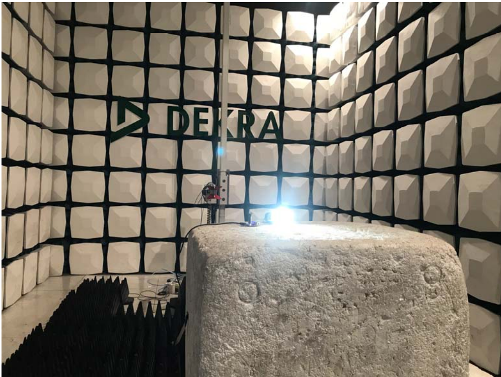
Description: Radiated Emission Test Setup for 1~18GHz
