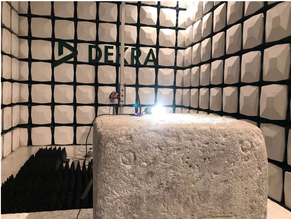
Description: Radiated Emission Test Setup for 1~18GHz
