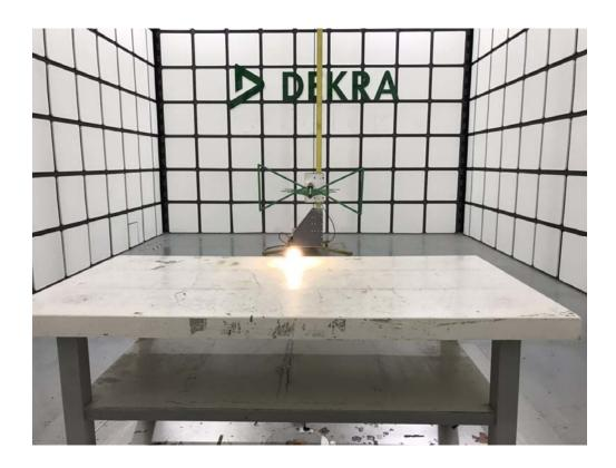
Description: Radiated Emission Test Setup for 1~18GHz
