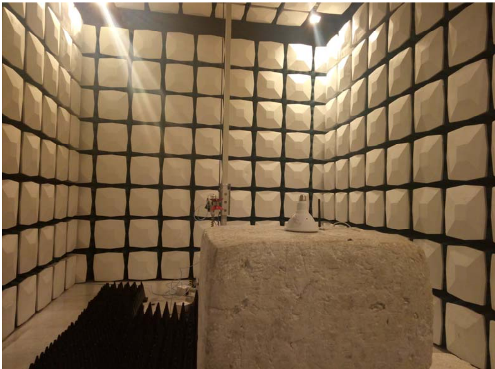
Description: Radiated Emission Test Setup for 1~18GHz
