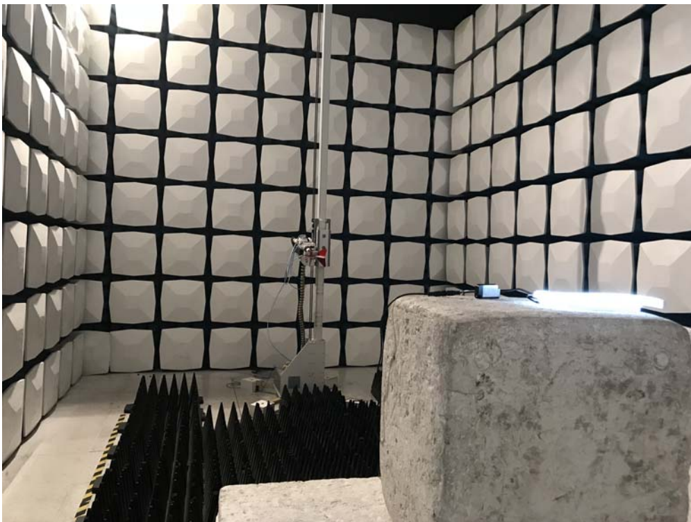
Description: Radiated Emission Test Setup for 1~18GHz
