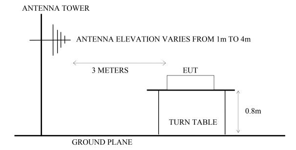
4.2.3. No. 1 3m Semi-Anechoic Chamber Setup Diagram (Test distance: 3m) for above 1GHz
