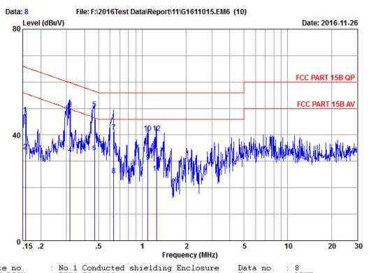
Site no. Limit Env. / Ins. EUT No.1 Conducted shielding Enclosure ESH2-Z5-1605 FCC PART 15B QP 20.6\*C&51%/ESCI LED Lamp 9290013015
