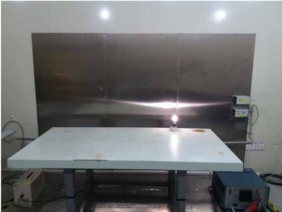
Front View of Conducted Disturbance Measurement
