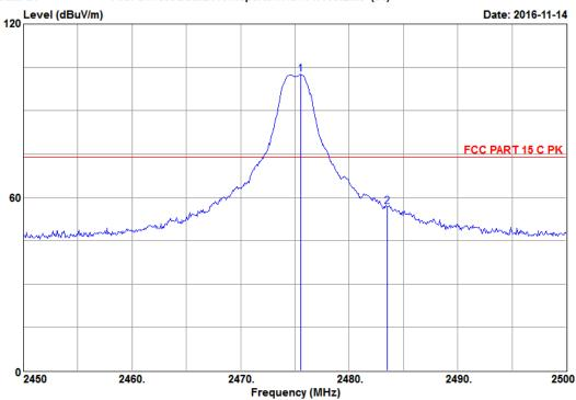
Site NO. : 3m Semi-Anechoic Chamber Dis. / Ant. : 3m 3115-62959-160620 Limit : FCC PART 15 C PK Env. / Ins. : 19.8\*C&58%/N9030A EUT : LED Lamp
