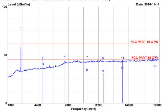
Site NO. : 3m Semi-Anechoic Chamber Dis. / Ant. : 3m 3115-62959-160620 Limit : FCC PART 15 C PK Env. / Ins. : 19.8\*C&58%/N9030A EUT : LED Lamp
