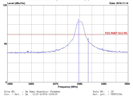
Site NO. : 3m Semi-Anechoic Chamber Dis. / Ant. : 3m 3115-62959-160620 Limit : FCC PART 15 C PK Env. / Ins. : 19.8\*C&58%/N9030A EUT : LED Lamp
