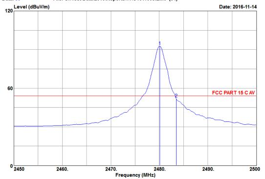
Site NO. : 3m Semi-Anechoic Chamber Dis. / Ant.: 3m 3115-62959-160620 Limit : FCC PART 15 C AV Env. / Ins.: 19.8\*C&58%/N9030A
