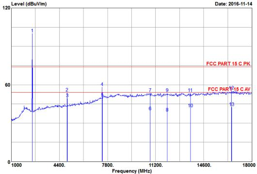
Site NO. : 3m Semi-Anechoic Chamber Dis. / Ant.: 3m 3115-62959-160620 Limit : FCC PART 15 C PK Env. / Ins.: 19.8\*C&58%/N9030A
