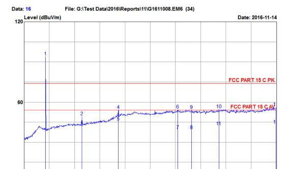
Site NO. : 3m Semi-Anechoic Chamber Dis. / Ant. : 3m 3115-62959-160620 Limit : FCC PART 15 C PK Env. / Ins. : 19.8\*C&58%/N9030A EUT : LED Lamp
