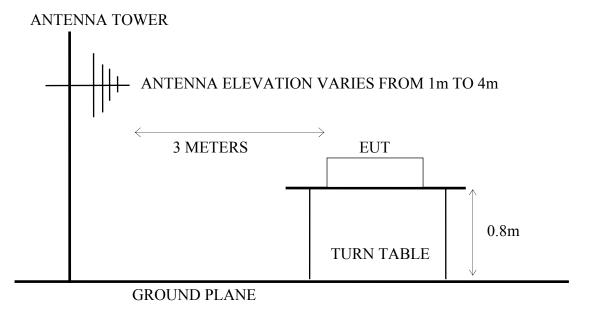
5.2.3. No. 1 3m Semi-Anechoic Chamber Setup Diagram (Test distance: 3m) for above 1GHz
