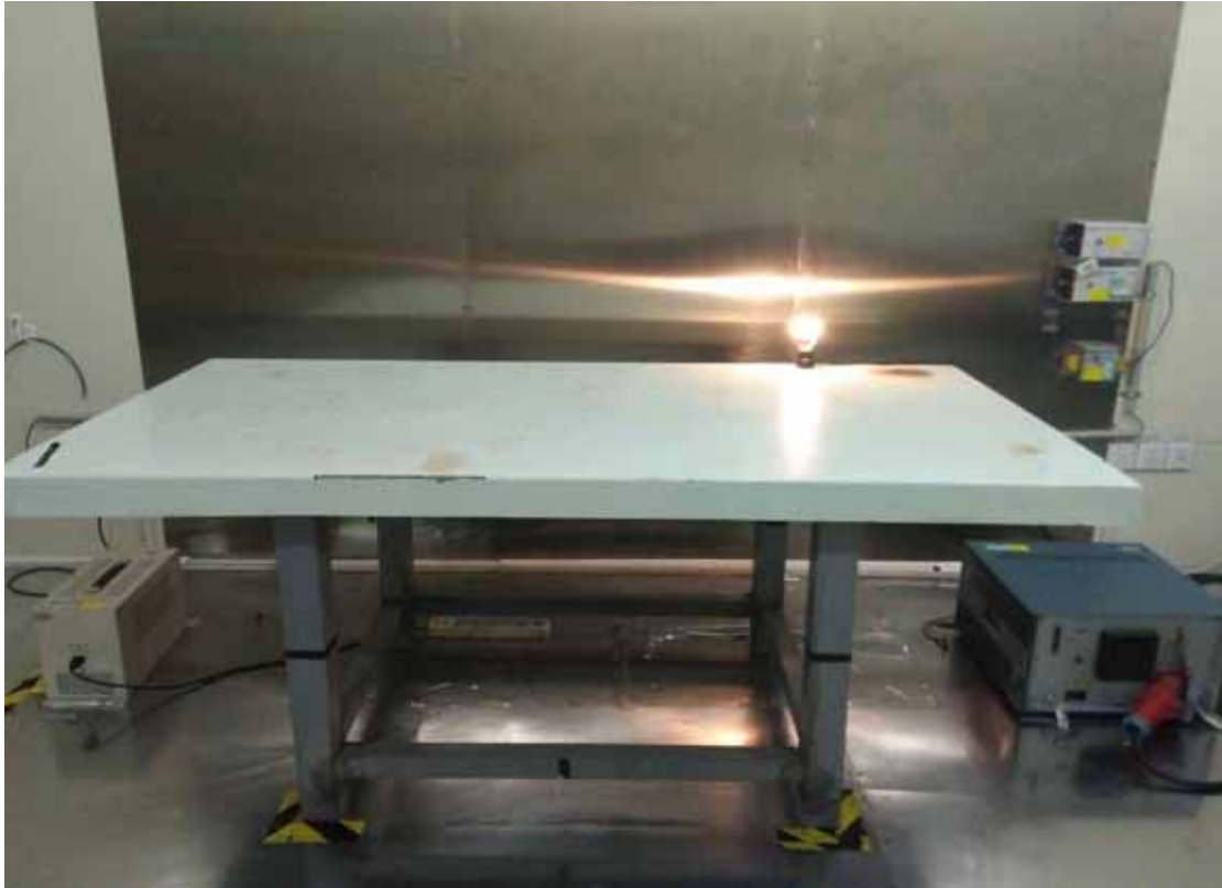
Front View of Conducted Disturbance Measurement
