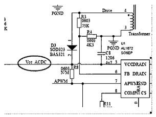
3. Add feedback circuit in RF board to limit the min. of VCC, see blue circuit.
