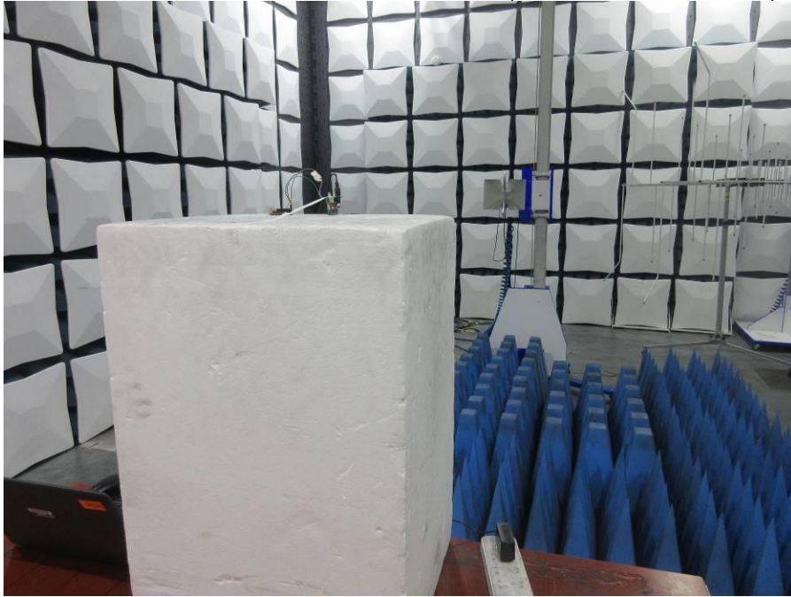
RADIATED RF MEASUREMENT SETUP (CLOSE SHOT)
