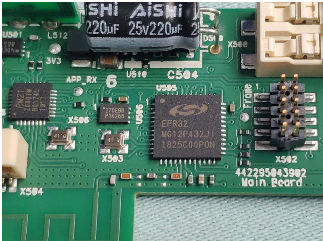
FIGURE 22 MISCELLANEOUS CONTROLS (M/N: SC1500/05) CHIP & CRYSTAL ON CONTROL BOARD (GENERAL VIEW)
