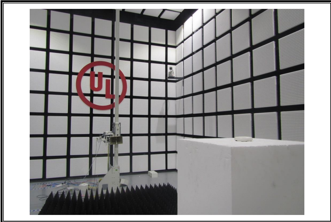
RADIATED RF MEASUREMENT SETUP (ABOVE 1 GHz)
