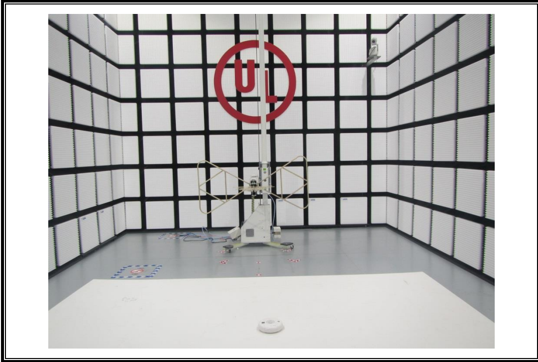
RADIATED RF MEASUREMENT SETUP (ABOVE 1 GHz)
