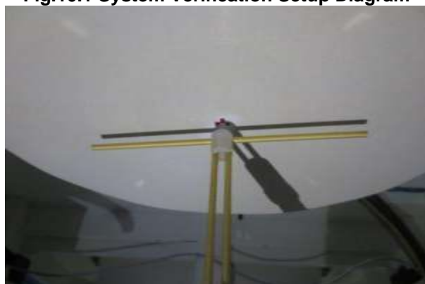
Fig.10.2 Photo of Dipole setup
