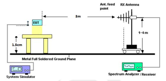
For radiated test from above 1GHz
