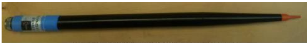
Figure 1 – MVG COMOSAR Dosimetric E field Dipole
