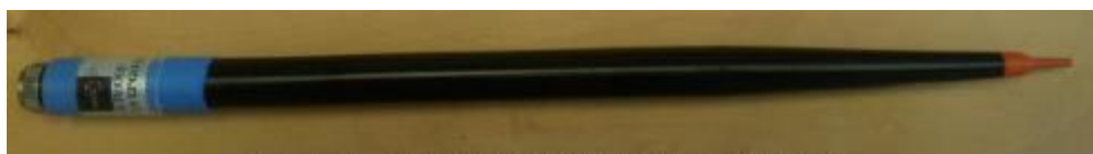
Figure 1 – MVG COMOSAR Dosimetric E field Dipole
