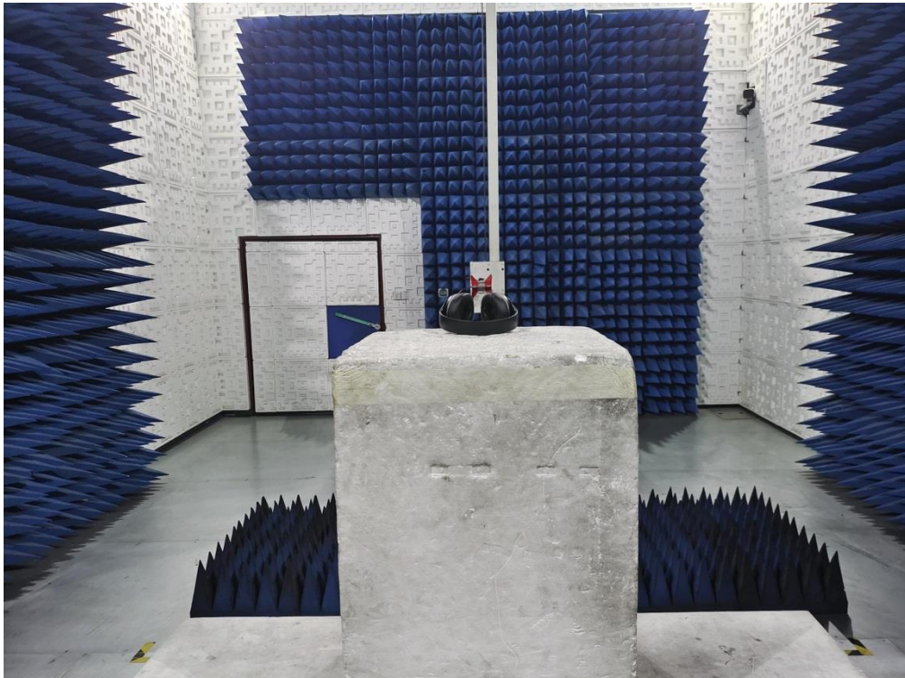
RADIATED EMISSION TEST SETUP ABOVE 1GHz
