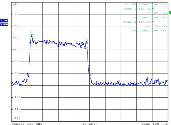
According the test data above, the fundamental wave is not fall in the restricted band 90KHz-110KHz and 0.495-0.505 MHz, the field strength also meets the 15.209 requirement, please refer to clause 7.3.
