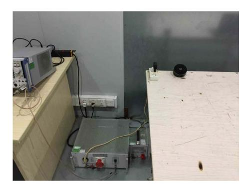
Radiation Emission Test Setup (Below 30MHz)
