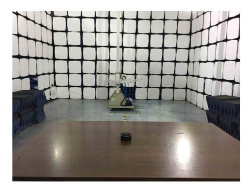
Radiation Emission Test Setup (Above 1GHz)
