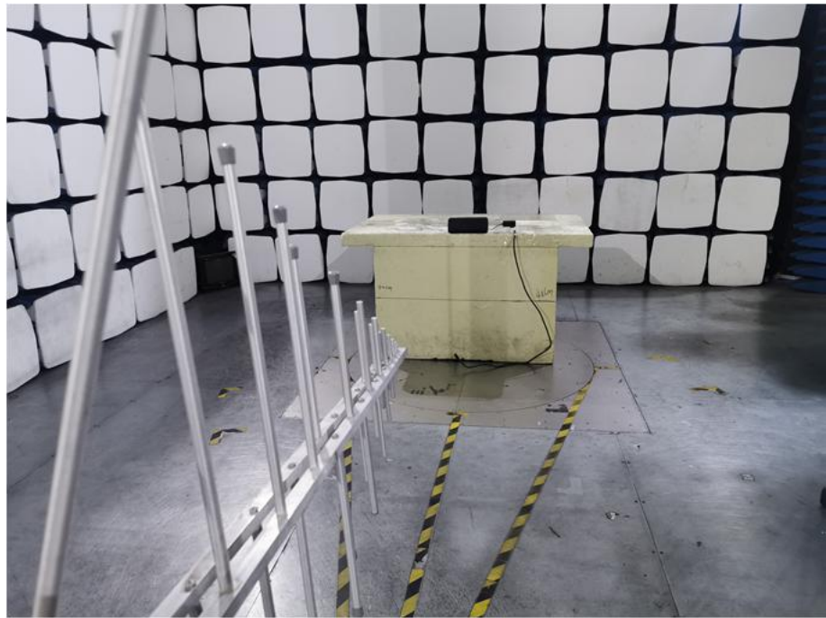
Radiation Emission Test Setup (30MHz to 1GHz)
