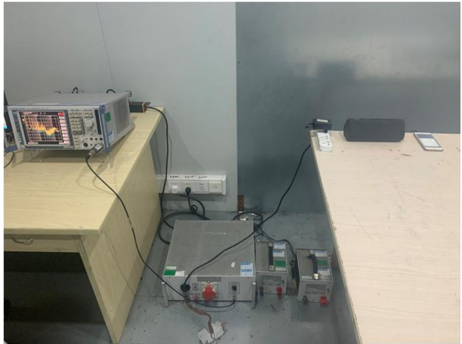
Conducted Emission Test Setup
