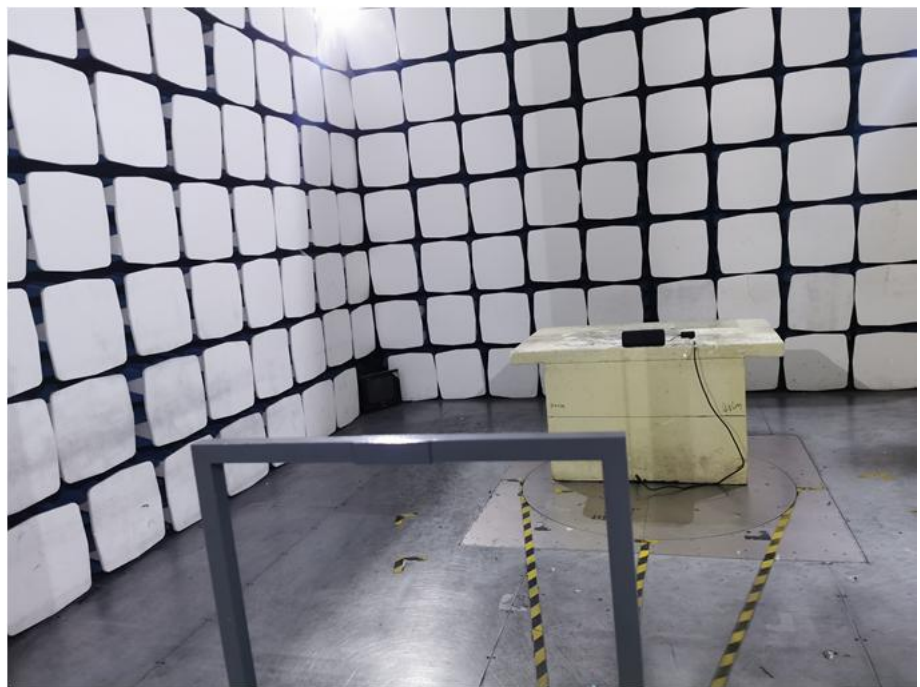
Radiation Emission Test Setup (Below 30MHz)
