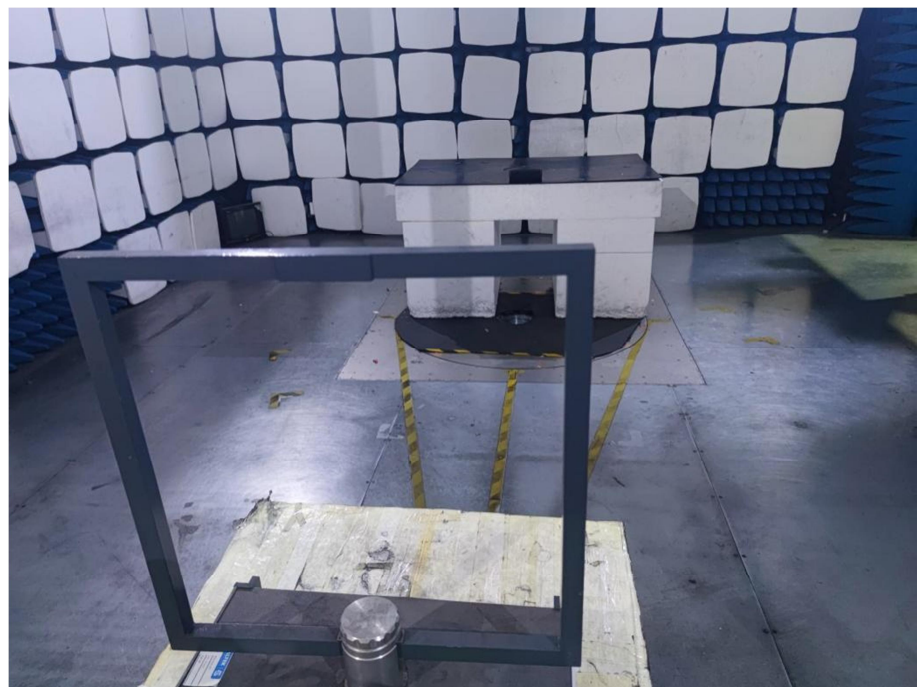
Radiation Emission Test Setup (Below 30MHz)
