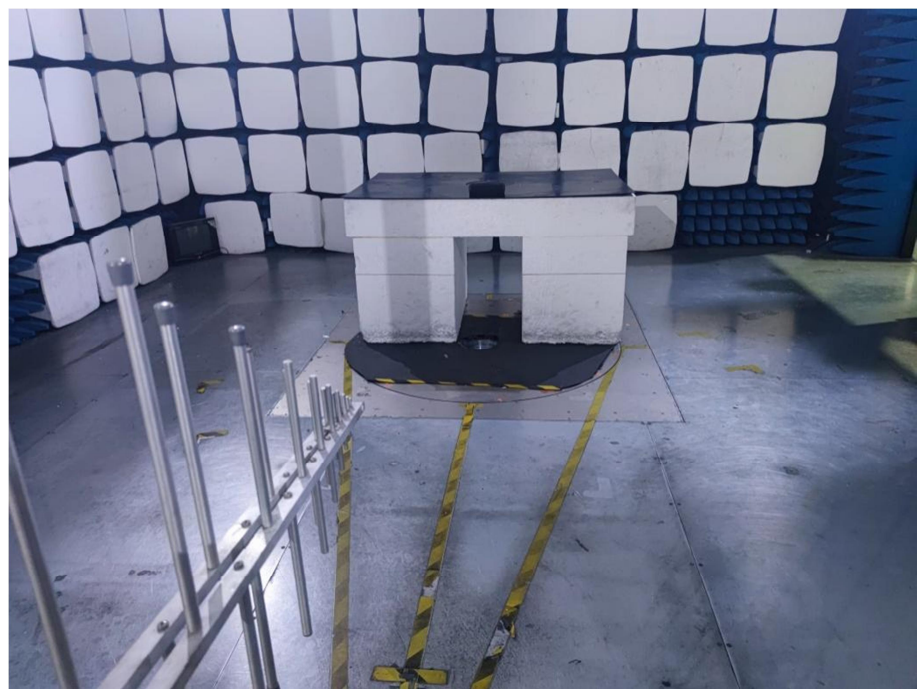
Radiation Emission Test Setup (30MHz to 1GHz)
