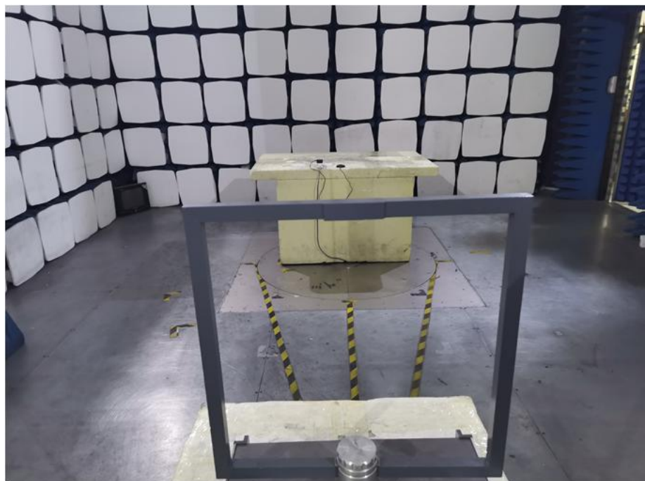
Radiation Emission Test Setup (Below 30MHz)
