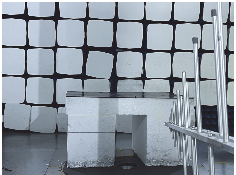
Radiation Emission Test Setup (30MHz to 1GHz)
