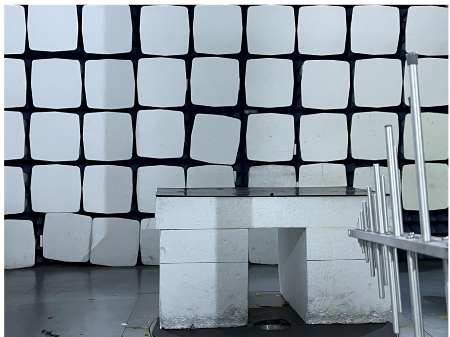
Radiation Emission Test Setup (30MHz to 1GHz)
