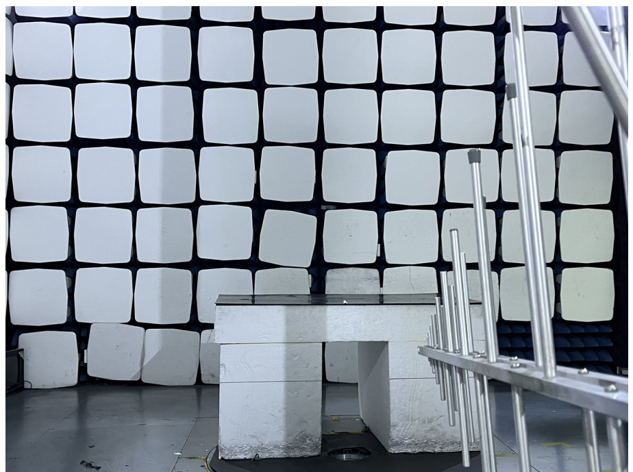
Radiation Emission Test Setup (30MHz to 1GHz)
