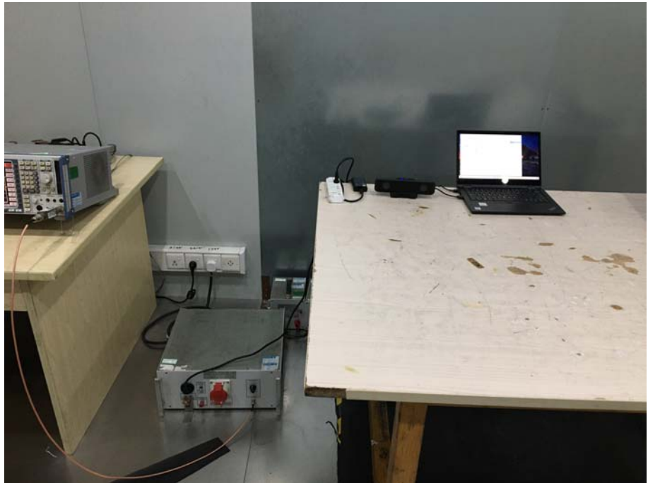
Conducted Emission Test Setup
