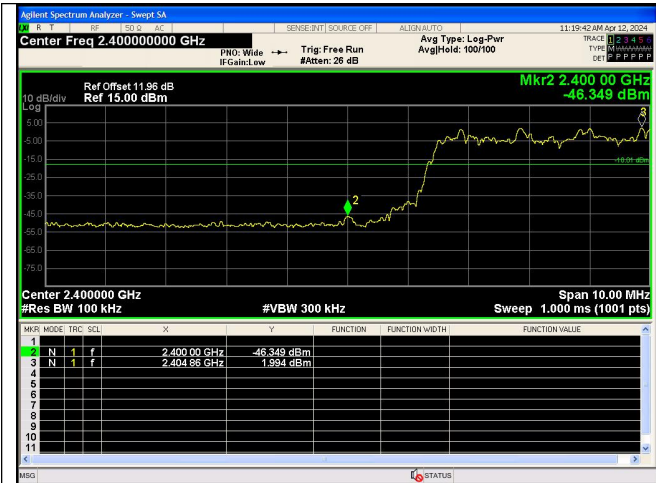
Out Of Band Emission(Left) 8DPSK_3-DH5_Channel Hopping
