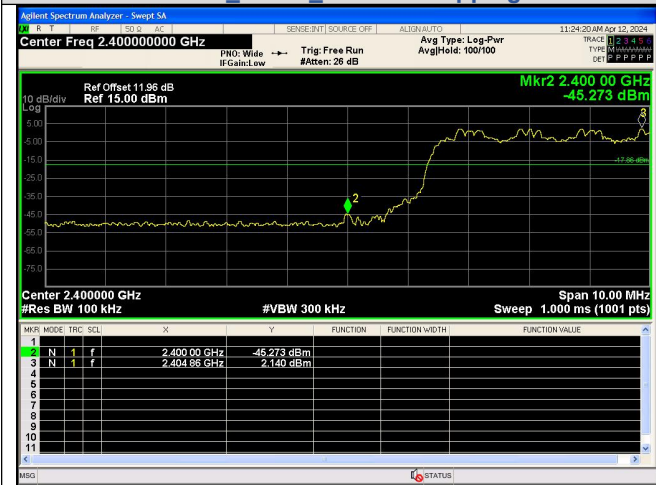
Out Of Band Emission(Left) 8DPSK_3-DH5_Channel Hopping
