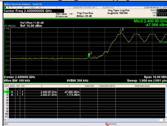
Out Of Band Emission(Left) GFSK_DH5_Channel Hopping
