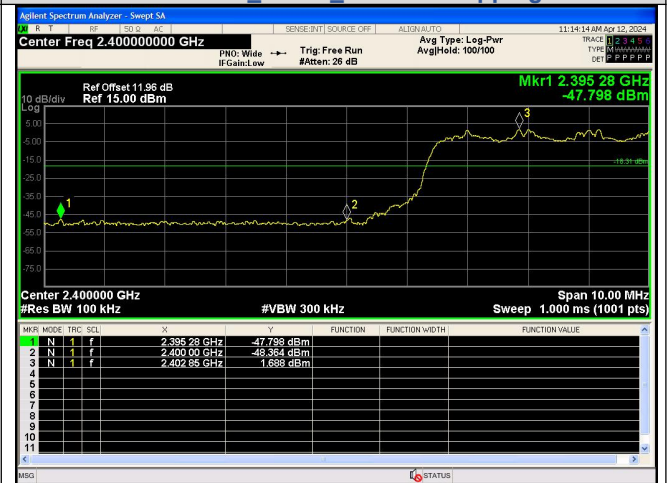
Out Of Band Emission(Left) \pi/4 DQPSK_2-DH5_Channel Hopping
