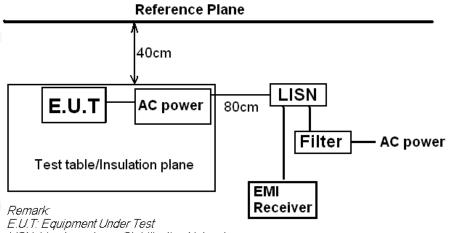
E.U.1: Equipment Under Test LISN: Line Impedence Stabilization Network Test table height=0.8m
