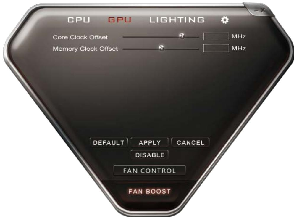
Core Clock Offset: Increase the upper threshold of the GPU clock and Boost clock.
