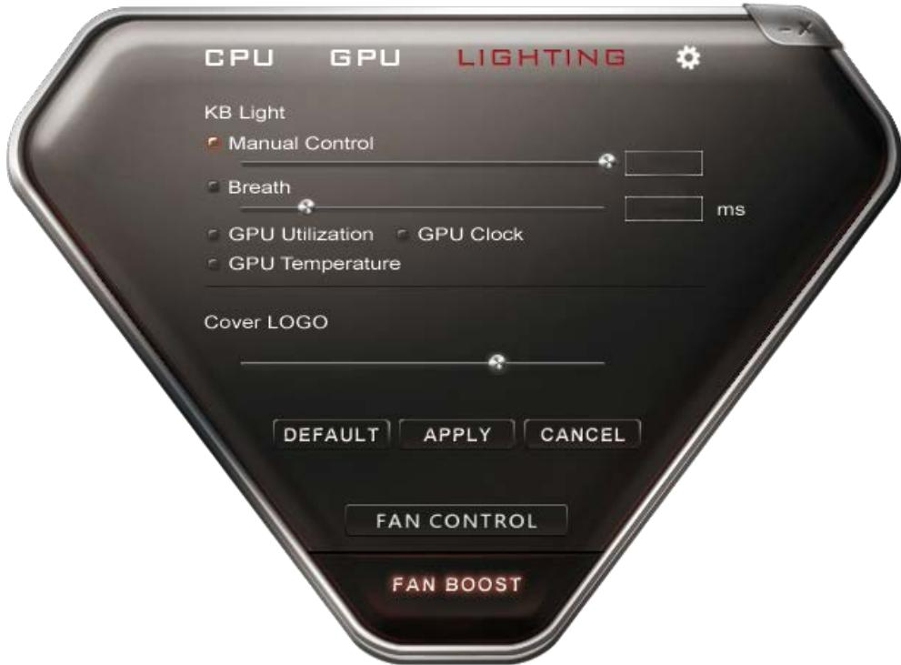
**Manual Control:** This slider gives you manual control over the brightness of the Keyboard backlighting.
