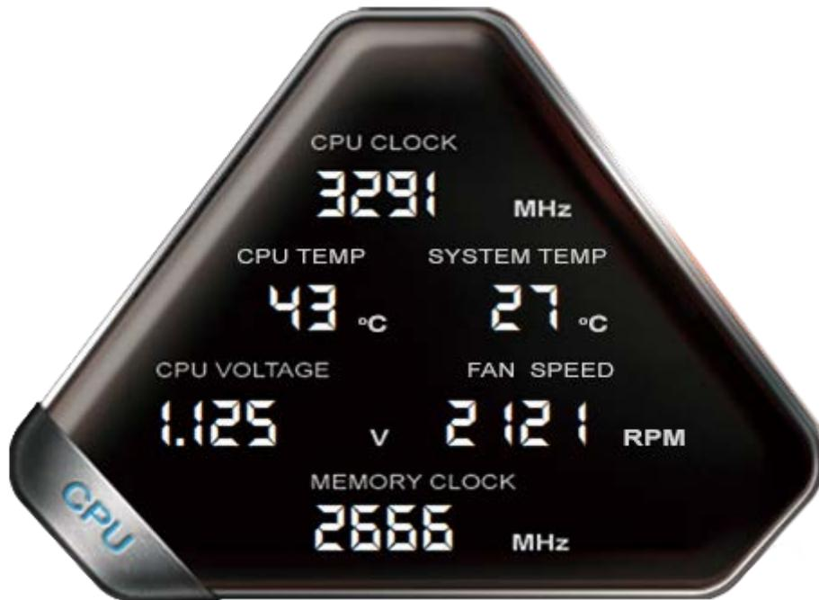
**CPU Clock:** This will show the current frequency of your CPU. The CPU frequency will vary based on load, background applications, etc. It is common, without overclocking, to see this specific model of CPU fluctuate between 800 MHz and 3900 MHz (3.9 GHz). Overclocking the CPU will change the frequency parameters, but the clocks will still fluctuate.
