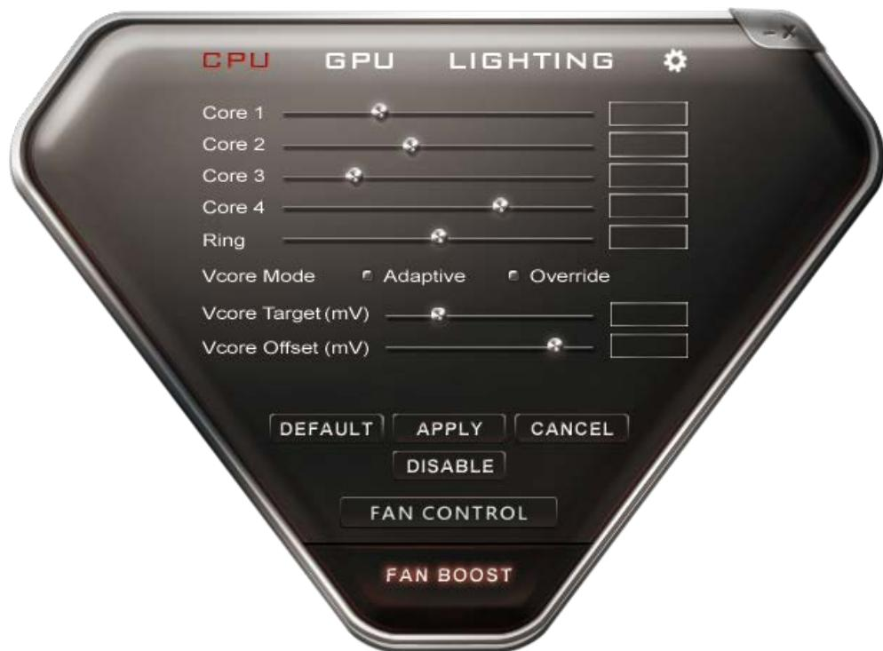
Core 1: Displays the current max multiplier for Core 1
