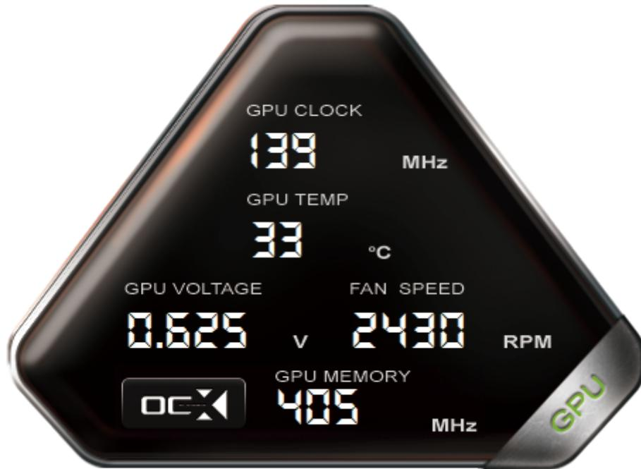
**GPU Clock:** This will show the current frequency of your GPU. The GPU Clock will vary based on load, background applications, etc.
