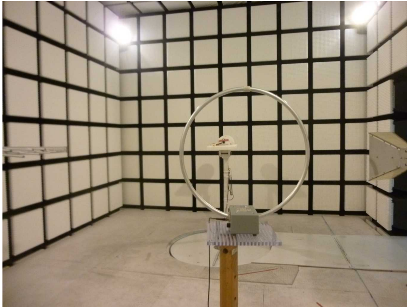
Photo 3: EUT at the anechoic chamber
