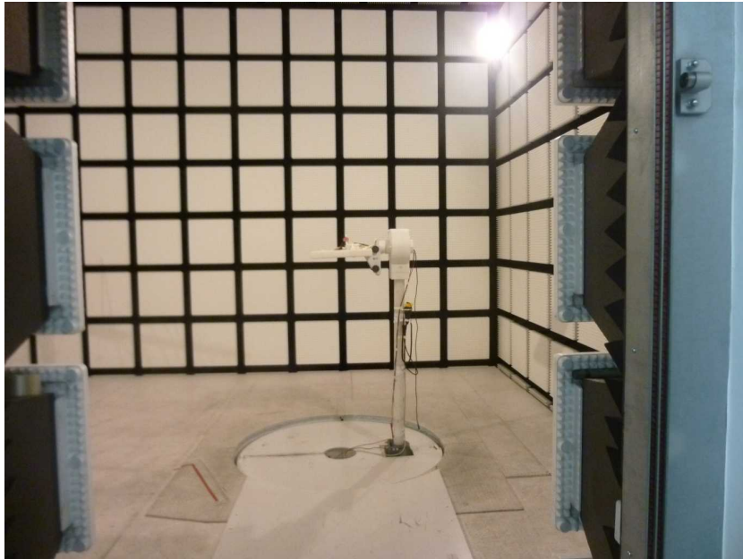
Photo 1: EUT at the anechoic chamber
