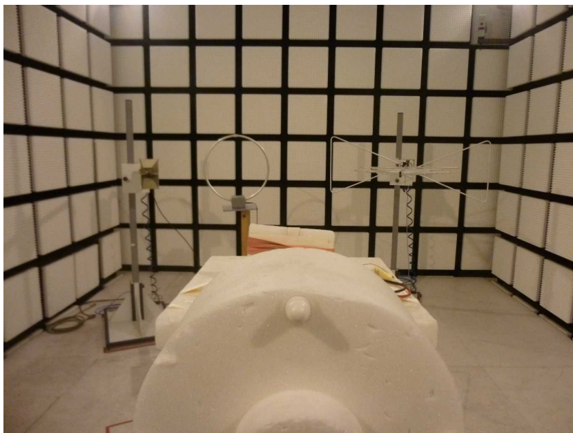
Photo 4: EUT at the anechoic chamber
