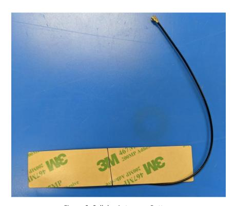
Figure 6: Cellular Antenna – Bottom
