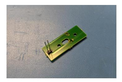
Figure 5: RFID PCB - Bottom
