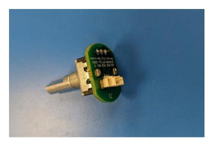
Figure 6: Encoder PCB – Bottom
