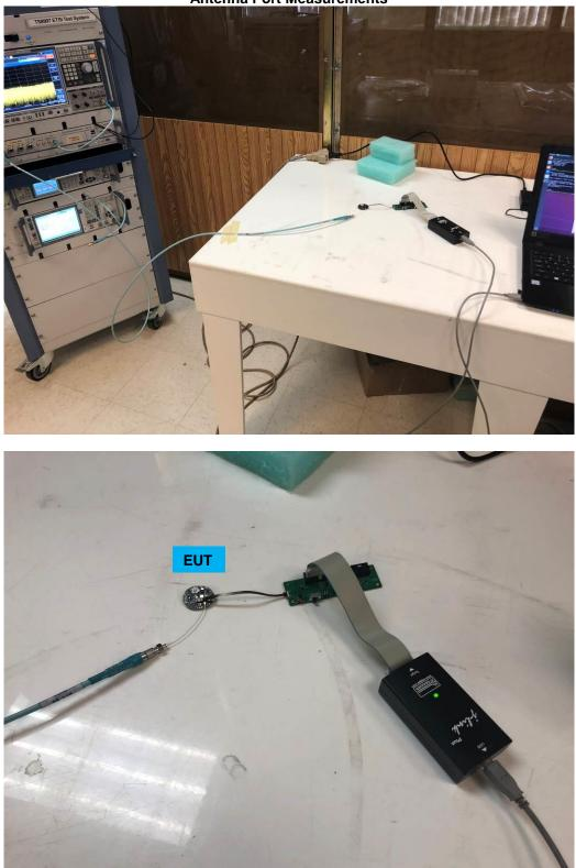
Radiated Emissions Test Setup, Above 1 GHz
