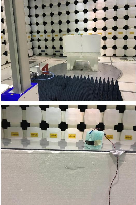
Radiated Emissions Test Setup, Above 1 GHz
