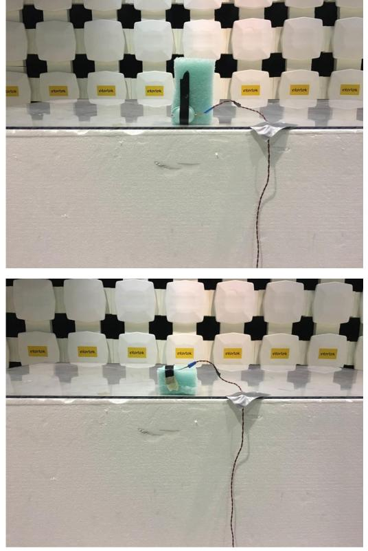
Radiated Test Setup, 30-1000 MHz
