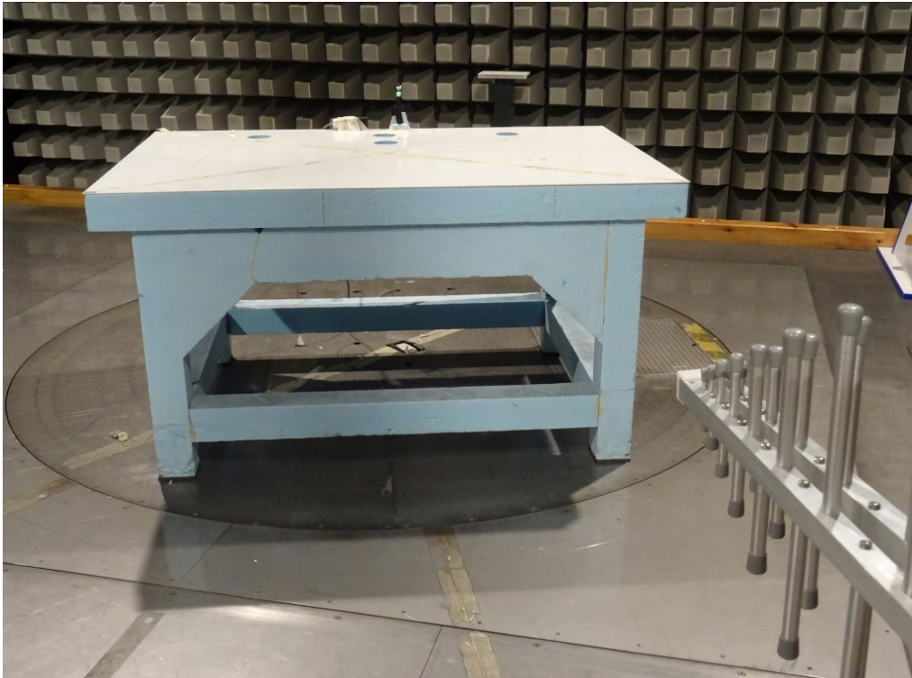
Test Configuration Photograph - Radiated emission below 1GHz.
