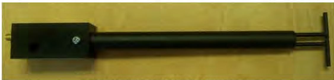
Figure 1 – MVG COMOSAR Validation Dipole
