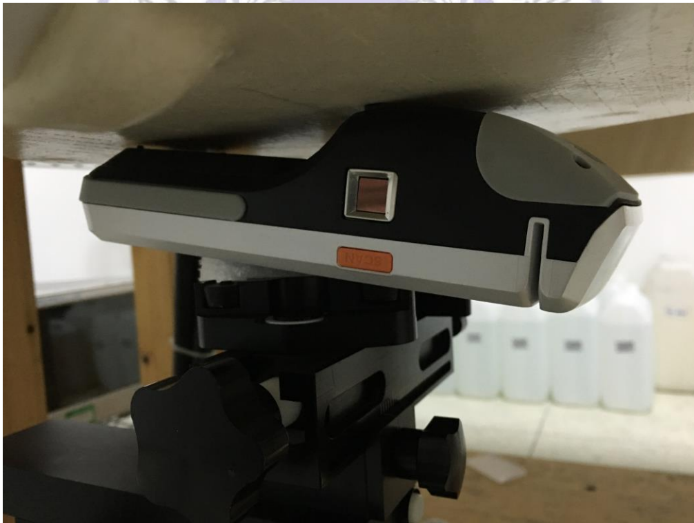
0mm Body-worn Accessory Rear Side Setup Photo
