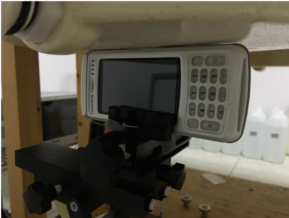
0mm Body mode Right Edge Setup Photo
