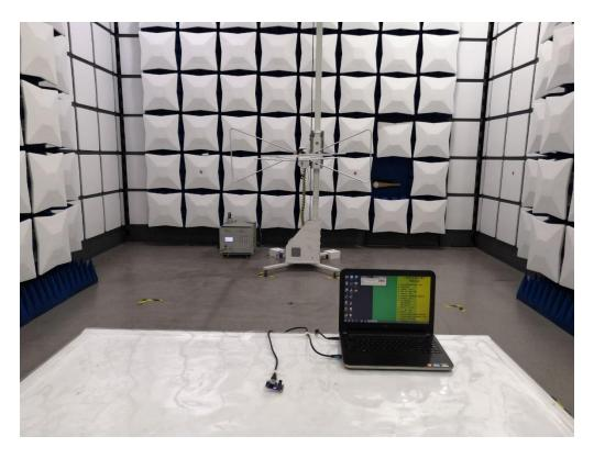
RADIATED EMISSION TEST SETUP ABOVE 1GHZ
