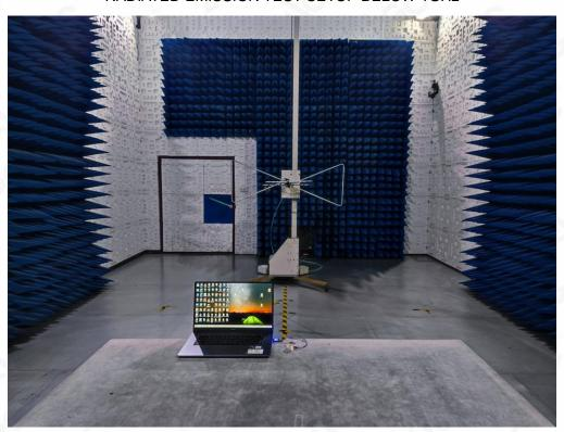
RADIATED EMISSION TEST SETUP ABOVE 1GHz
