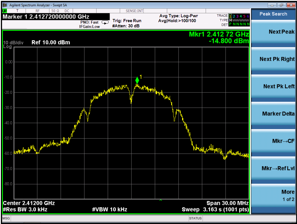
802.11b TEST RESULT TEST PLOT OF SPECTRAL DENSITY FOR LOW CHANNEL
