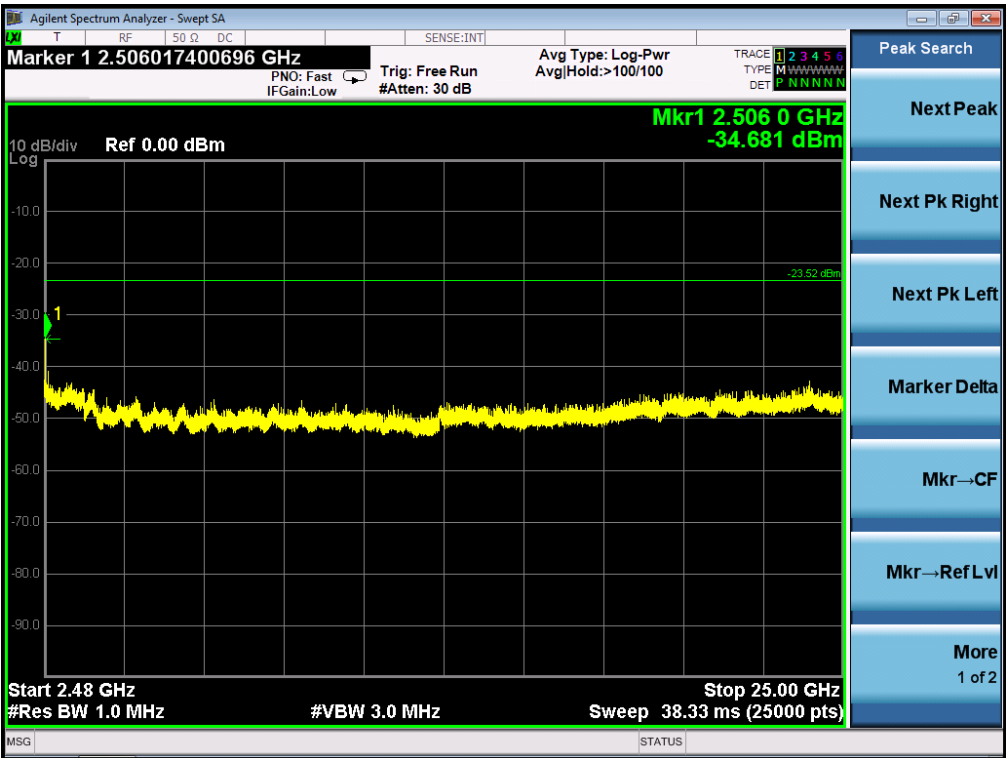
TEST PLOT OF OUT OF BAND EMISSIONS THE WORST CASE OF 802.11g FOR MODULATION IN HIGH CHANNEL
