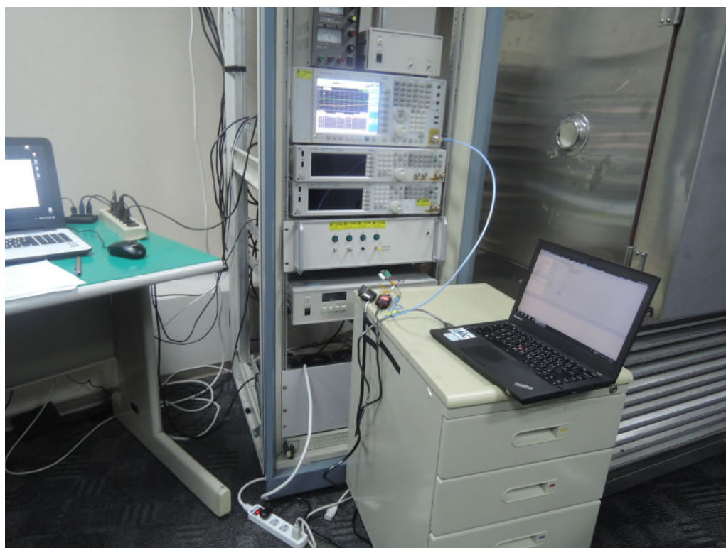
Photograph 7: Set-up for Conducted testing
