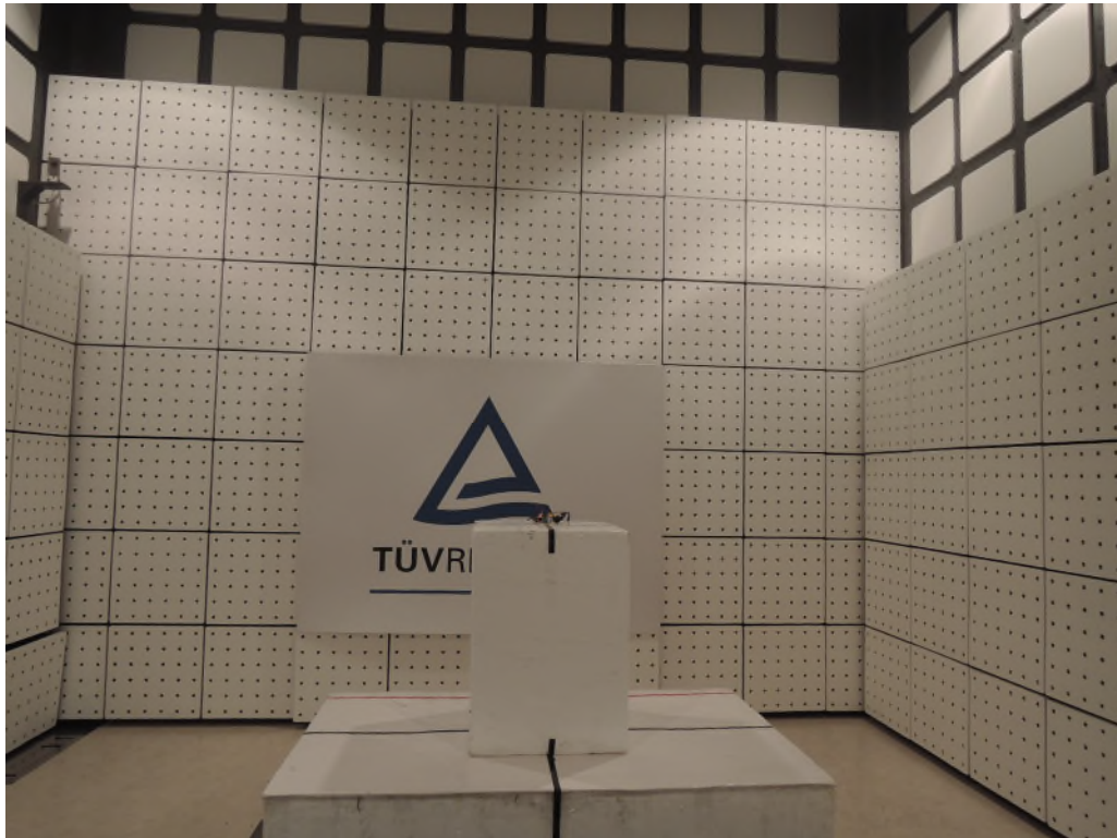
Photograph 3: Set-up for Spurious Emissions (Back View 1)
